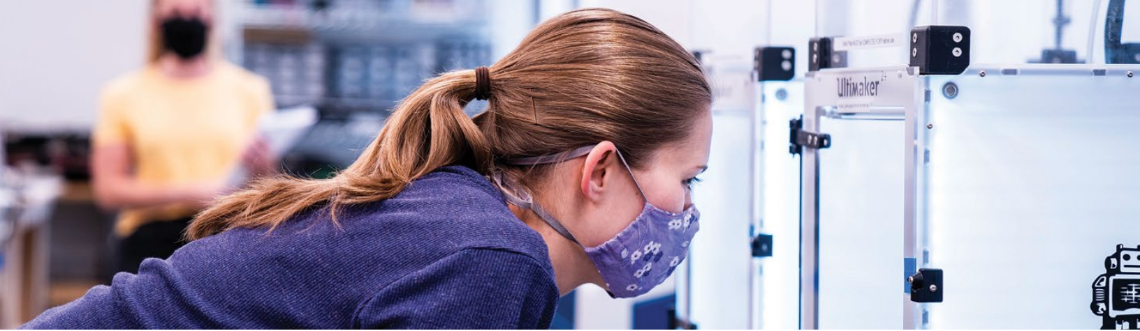
Sara Willman, lab manager at UCI Beall Applied Innovation, utilizes a fused deposition modeling 3D printer, which uses continuous filament of thermoplastic material, to make a sign for Applied Innovation's lobby.
