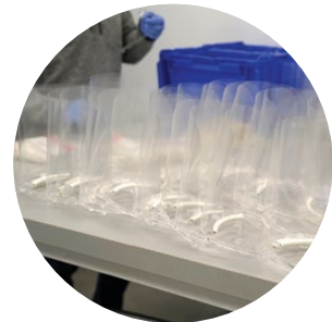
Elastic straps are attached after the transparent shields are added.
