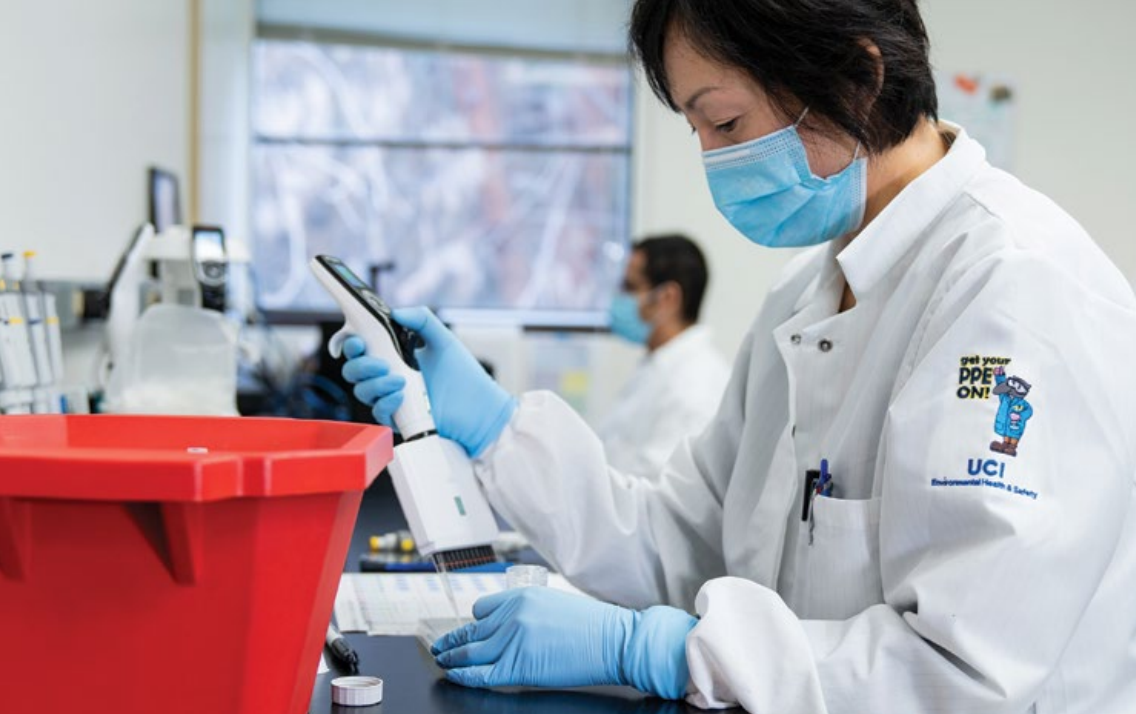
Rie Nakajima, Ph.D., lab research supervisor, is using a pipette to put proteins onto source plates, which will go into the microarray printer in the Protein Microarray Laboratory and Training Facility at UC Irvine's Institute for Immunology.
